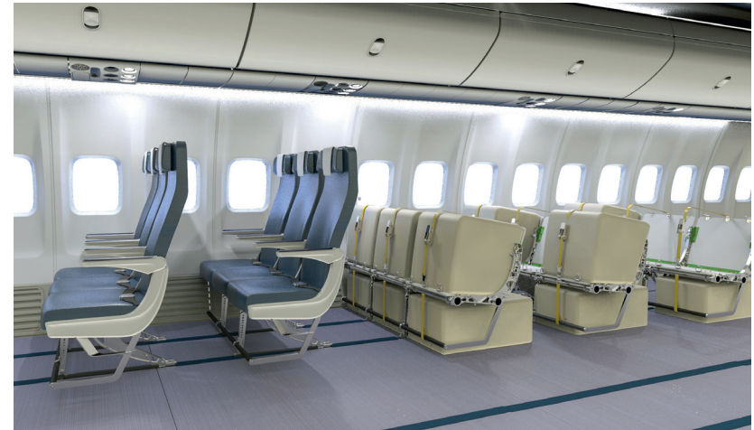
Passenger aircraft interior stowage devices developed by HAECO Cabin Solutions, offering airline customers solutions to combine passengers and cargo in main cabin during the COVID-19 pandemic.
